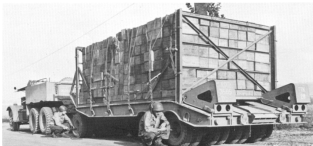
TRACTOR-TRAILER COMBINATIONS used on the Continent: 4-5-ton, 4 x 4, truck tractor, COE, with 2,000-gallon gasoline semitrailer, top; 1 1/2-ton, 4 x 4, truck tractor with 3 1/2-ton stake and platform semitrailer, center; 12-ton, 6 x 4, truck with 45-ton trailer (tank transporter), bottom.
